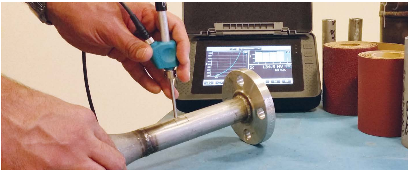
Figure 26: Performing Leeb measurements on test sample
