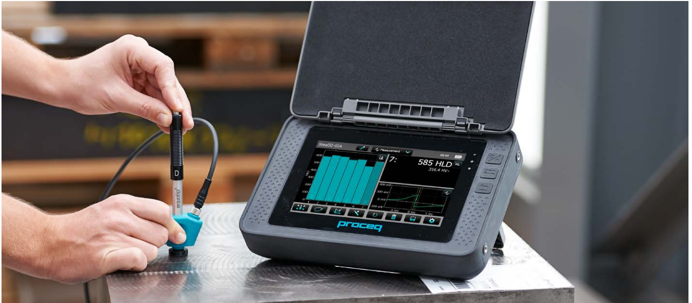
Figure 5: Equotip 550 Leeb hardness testing instrument
